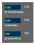
With the controller in automatic mode, observe behavior for step changes in set point above and below the steady-state value. Comment on your observations in your report. Tune the controller by adjusting the constants to improve performance.
