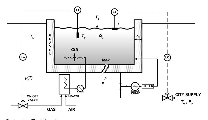
Outputs:  $T_p$ , L(level) Inputs: Q(t),  $F_w$ Disturbances:  $T_w$ ,  $T_a$  $Q(t) = UA(T_p - T_a) + k_G \frac{(T_p - T_G)}{\Delta x} + F_w \rho C(T_p - T_w)$
