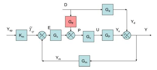
Derive a dynamic and static feedforward controller ( $G_{ff}$ ) that will best reject the disturbance (D).
