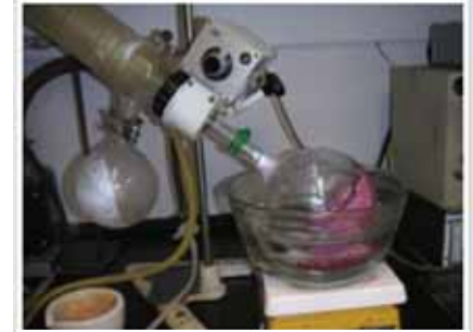
Preparation of FT Cobalt Catalyst
